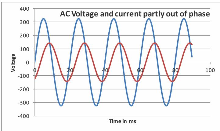
Figure 8: AC voltage and current with a partly inductive load
