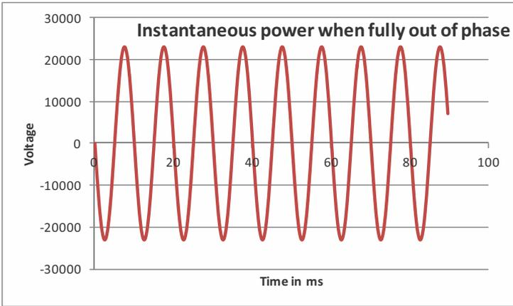
Figure 7: Instantaneous power in a purely inductive load AC load
