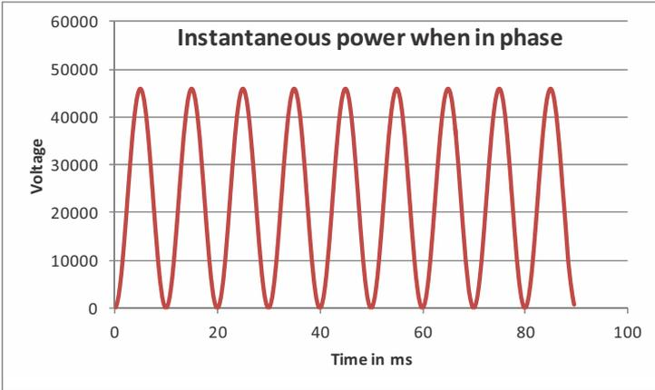
Figure 5: Instantaneous power in a resistive AC load
