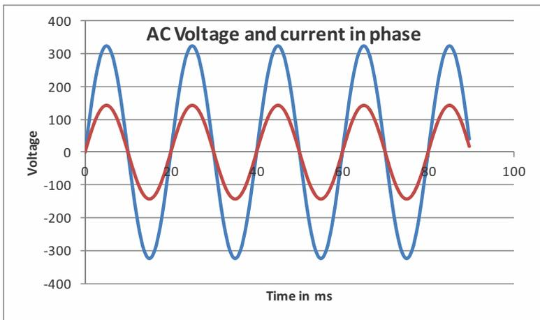
Figure 4: AC voltage and current with a resistive load (in phase)
