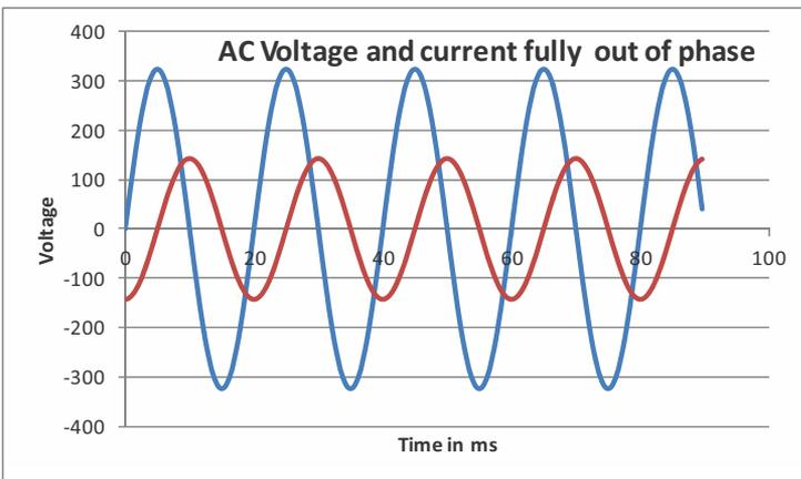
Figure 6: AC voltage and current with a purely inductive load
