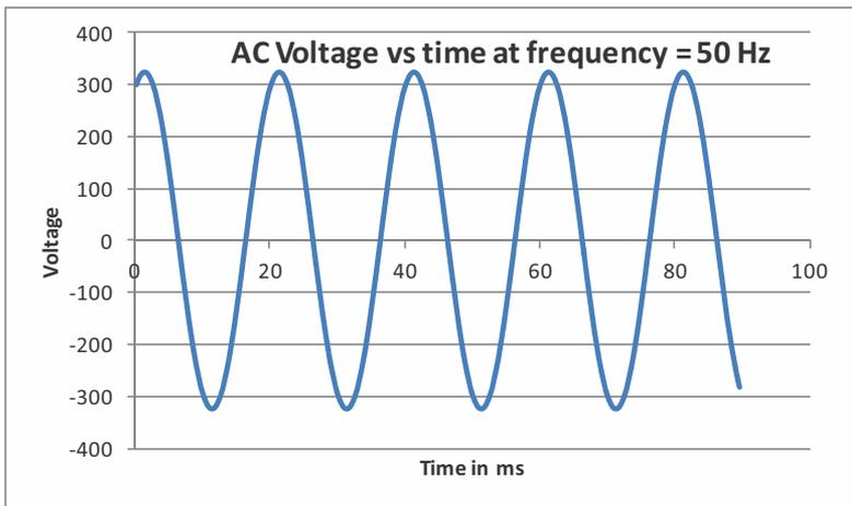
Figure 2: oscillating voltage in an AC circuit at 50 Hz
